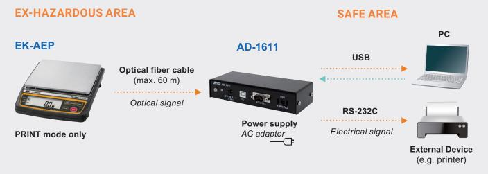
\*When the AD-1611 is connected to a PC via USB, power is supplied from the PC. When the RS-232C is used, power needs to be supplied from the AC adapter. Only a PC can be connected to the USB port of the AD-1611. 1 m USB cable type B male - type A male is included
